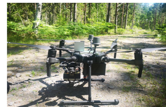
Drone with multispectral sensors acquiring precise imaging of crown conditions in disease-stricken stands.
