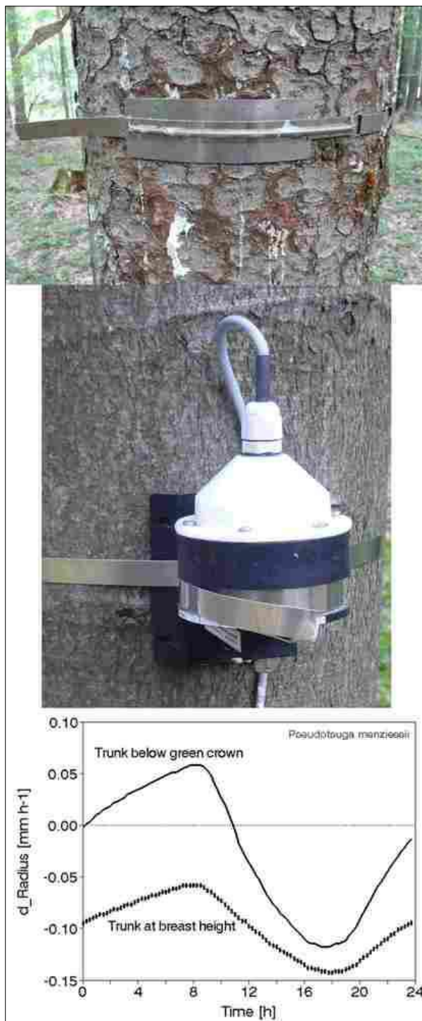
Fig. 35 - Usual band dendrometer for periodical manual reading of trunk circumference based on nonius scale, which is suitable for seasonal recording of stem growth (step 0.1 mm - upper panel). Electronic dendrometer measuring stem circumference (intermediate panel). Diurnal changes of stem radius measured with the electronic, especially sensitive dendrometer continuously recording similar data below green crown and around breast height (lower panel).
