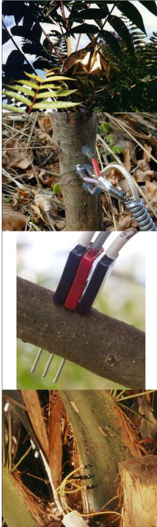
Fig. 28 - Sap flow meter based on the THB method with external contact heating installed on the petiole (5 mm in diameter) of a large leaf of Ailanthus glandulosa (top panel). Sap flow meter based on the HFD method installed on the small (25 mm in diameter) stem of Fagus sylvatica sapling (second panel) and in the branch by the heat ratio method (HRM) (third panel). Thermometers are switched off in that part of needles, which are outside the measured stem. Sap flow measurement by the multipoint HFD sensor in the large leaf of palm (fourth panel), where most flow goes through its center.
